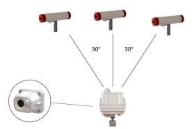
**4.** Make similar tests from various locations within the protected area, the detector should respond as stated above. **NOTE:** The portable UV Test unit is designed to check for operation only, not for precision sensitivity testing. This must be accomplished at Firefly AB.
