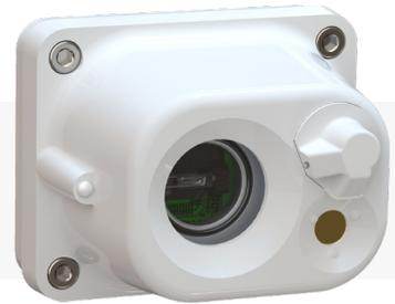
The Omniguard® model 860 UV/IR flame detector is designed to detect fires and output appropriate alarm information. The model 860 senses ultraviolet radiation and infrared radiation in the appropriate wavelengths for very early fire detection. Using the patented Fire Event Analysis (FEA) algorithm, it is also able to distinguish between real fire and non-fire events providing superior false alarm immunity. The technology has proven itself over decades of reliable service.
